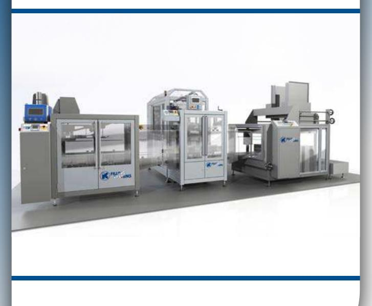
Automatic line for filling and packaging liquids in Bag in Box packs
