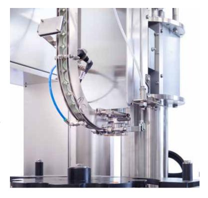
Italian made quality in an automatic rinser / filler / seamer with low oxygen pick up **New** EPV counterpressure electro-pneumatic filling valves for extended shelf life
